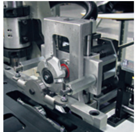
75 mm cutters with shaped profile (2 mm radius)
