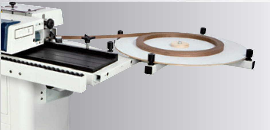
730 mm diameter coil holder plate with side limit rollers
